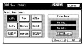
6 Specify the adjustment for moving the printing position up and down and to the left and right.
